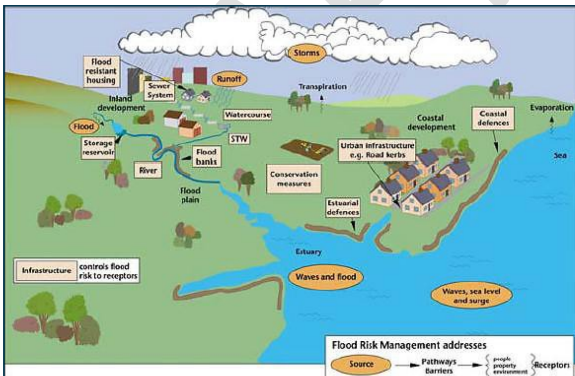
Figure 5.3: Source-pathway-Receptor Model for Flood Risk Analysis (source: Foresight Flood and Coastal Defence Project, 2003)
